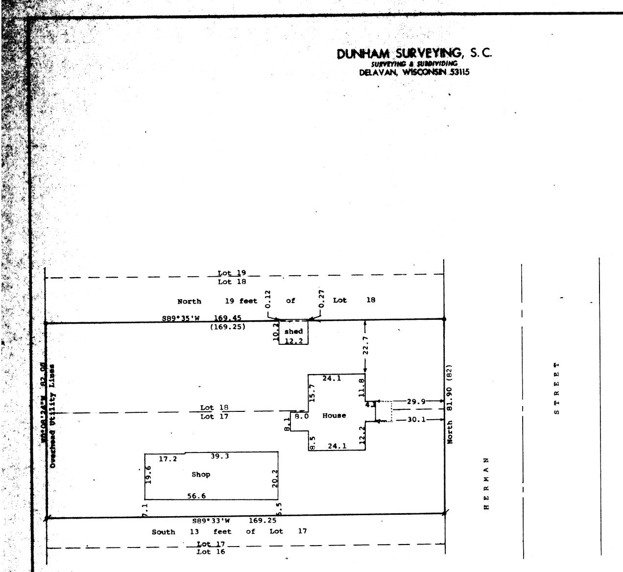
Scale - 1" = 20ø = ⅓" Iron Pipe Found 0 = 3/4" Iron Pipe Found • = 14" Iron Pipe Found Bearings referenced to the assumed bearing of North along the west line of Herman Street Survey ordered by: Donald E. Erdman 516 Herman Street Delavan, WI 53115 (0.00) = Recorded distance
